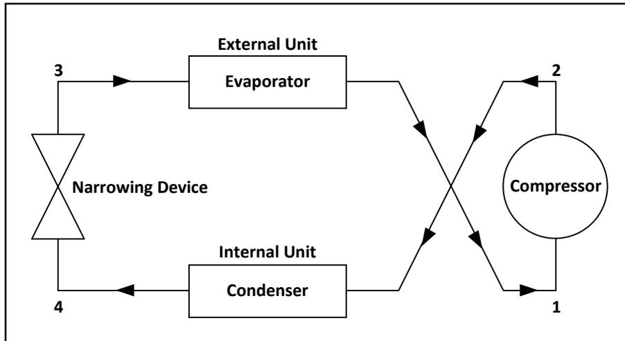
**Figure 2-1 Reverse thermal cycle**
