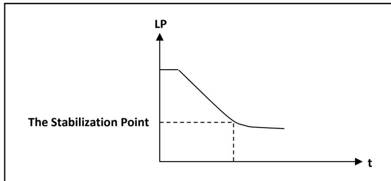
At the stabilization point the suction pressure (LP) is almost unchanged.
